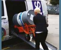
Specifically designed lightweight two piece ramp that will fit onto most types of van is easily transferable to vehicle allowing higher delivery fleet flexibility.
